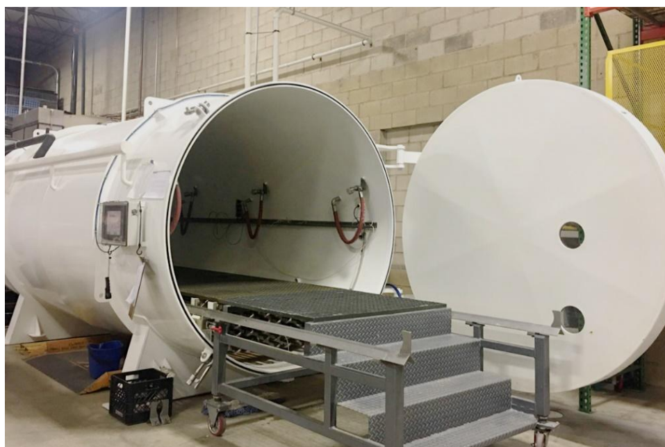
Figure 3. Ma, Y. (2020). Polygon's chamber for freeze-drying artifacts, 2020. Retrieved from https://user-images.githubusercontent.com/47676628/89826840-d3fb7880-db24-11ea-94d1-e4d8d62f5bbf.jpg
